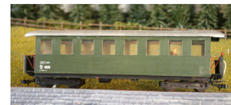
A bogie coach conversion based on Fleischmann Magic Train coaches
