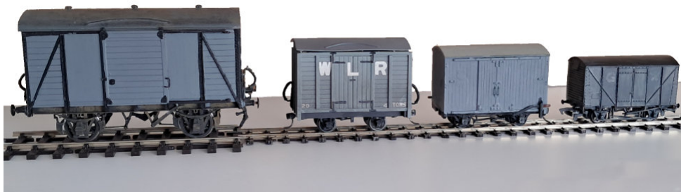
A comparison of Scale and Gauge. From left to right: standard O scale van on 32mm track; O-16.5 van on 16.5mm PECO narrow gauge track; On30 van on the same PECO track; a standard OO scale van on 16.5mm gauge OO scale PECO track.
